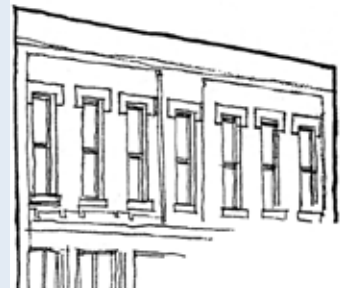
Existing building with missing cornice.
